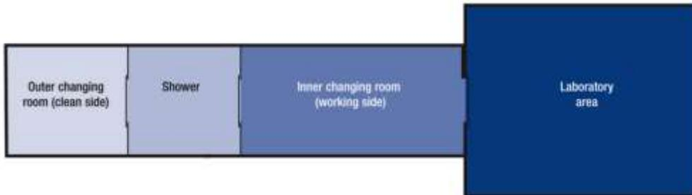
Figure 3. The typical design of a cabinet line BSL4 laboratory [3]
