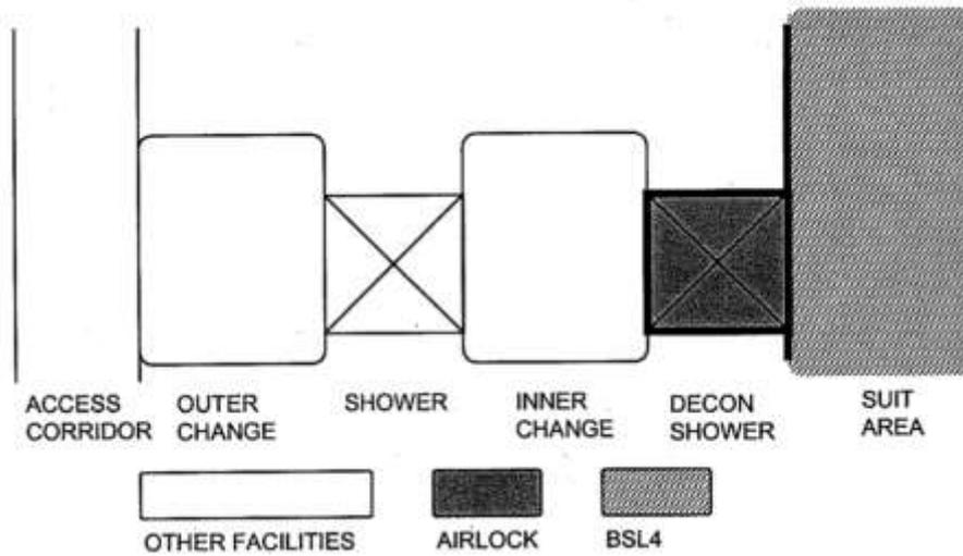
Figure 4. The typical design of a suited BSL4 laboratory [5]
