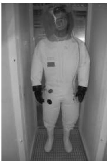
**Figure 1.** Worker within a positive pressure suit (Picture credit PHE).
